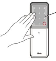
Touch the black screen once. The number will be displayed. Enter the PIN to unlock the device.
